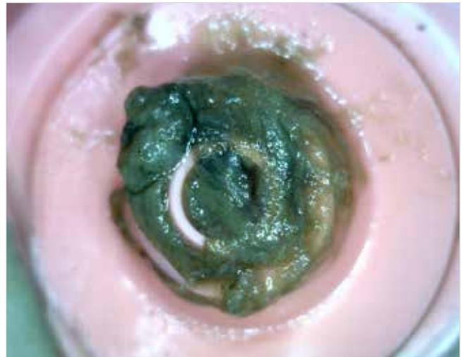
9. Algae build up causing dripper blockage
